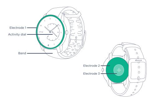
By placing the opposite hand on the watch, the user creates a closed electrical circuit with the arms and chest, allowing the measurement of a one-lead ECG.
